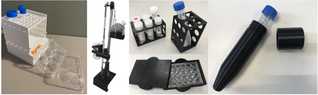
Figure 2. Examples of 3D printed lab equipment. Modular rack (left). Fluorescent camera holder (middle). Multi-function racks and dark equipment for fluorescent staining (right).
